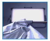
Insert poles into the pole sleeves on the Octa Lightbank. Ensure that the shorter smooth ferrules are inserted into the Lightbank. The longer, notched ferrules should be exposed.
