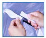
With the Lightbank on the fixture, attach the internal baffle to the white hook and loop tabs on the inside of the Lightbank.
