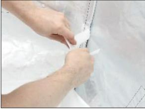
With the Lightbank on the fixture attach the internal baffle to the white hook and loop tabs on the inside of the Lightbank.
