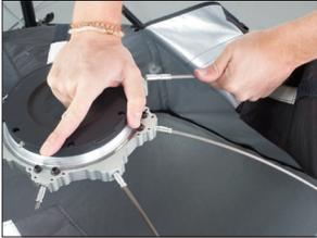
Insert poles into the pole holes on the Chimera Orbiter Speed Ring. Note that the tension on the Lightbank will become greater after inserting each pole. It may feel like you will break a pole, but you will not!
