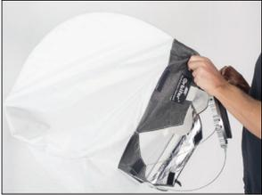
With all four wires inserted in the Speed Ring, pull the fabric over the wire, ensuring the wires line up with the seams.
